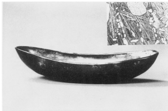
Fig. 4. Oval bowl of high-tin bronze. Iran, 7-8 century A.D. Made by hot forging, followed by quenching in water. Unlike steel, this alloy (22 per cent tin) is brittle if slowly cooled. (Metropolitan Museum of Art, Dr. Peter Meyers, Rogers Fund 1949). (Above) Microstructure of an Iranian bowl similar to that shown. The needle-like features are sections of plates resulting from a crystallographic change that occurred during rapid cooling. Etched. Magnified 500 times.
